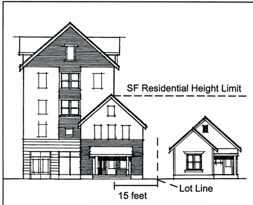
Figure 4-6 Residential Building Height Buffer
